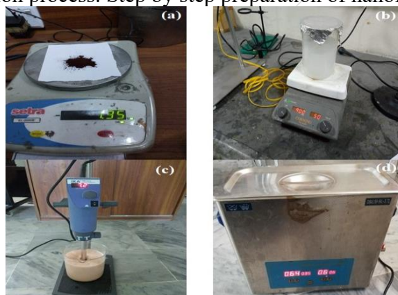
Figure 1: Nanofluid preparation (a) Weighing nanoparticles (b) Magnetic stirring (c) shear homogenization (d) Ultrasonication
